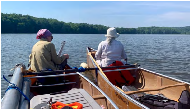
Fig. 3. Canoes lashed together will drill rods form the portable coring platform
