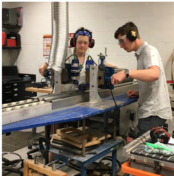
Fig. 5 Amy Myrbo, Ph.D. and Rob McManus splitting core tube with a vibrating medical cast saw during a training workshop.
