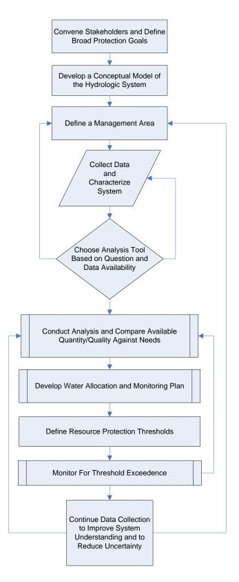
Figure 1. Process diagram for developing a sustainable management plan for groundwater.
